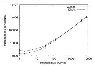
Figure 7: The request overhead of the wedge as a function of request size.
