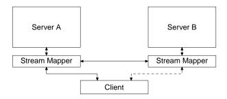
Figure 1: Failover architecture for a support group of two servers.
